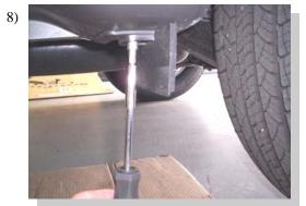
Remove the small stone protector that is in front of the rear wheel. This will not be reused.
