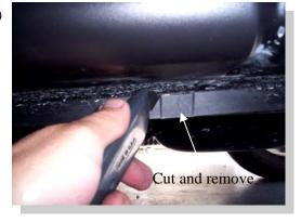
Measure from front wheel well back and make a mark at 11 1/2" (13" on passenger side), 26", 43" and 59". At each mark, remove about a 1-1/4" wide piece of the cladding covering the pinch weld.
