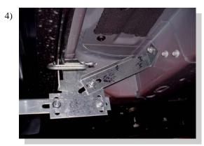
Assemble FL123 to BT54 as shown. Using a 5/16" bolt and nut attach the bracket to the pinch weld and the BT54 to the body using the bolt removed in step 3.
