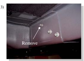
On the drivers side at the 11 1/2" location remove the upper bolt shown on the vehicle frame. <u>Do not discard.</u>
