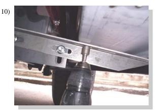
Set the board on the brackets and level. Make sure the board is centered between the wheel wells and is aligned evenly down the side of the vehicle Tighten the brackets to hold the board in place. Attach the board to the brackets with 3/4" long self drilling screws.
