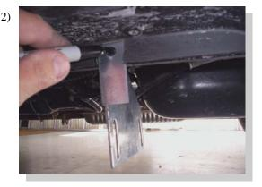
At each of the locations from step one, hold a bracket up and mark the center of the hole. Remove the bracket and drill a 23/64" hole through the pinch weld.
