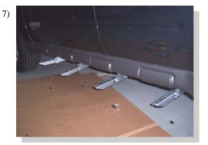
Attach one 3124F to each bracket with 5/16" bolts and nuts. Snug but do not tighten at this time
