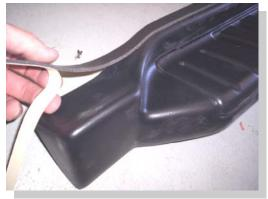
Install step tread and foam tape to the board.
