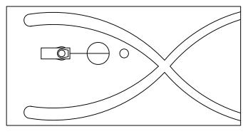
MOUNT BRACKET ASSEMBLY TO THE BODY WITH \$\frac{1}{16}\cong^{\text{"}} BOLTS AND NUTS THROUGH HOLES IN THE PICH WELD AND \$\frac{1}{16}\cdot^{\text{"}} BOLT INTO THE CLIP NUT OR 8MM BOLT INTO FACTORY NUT.
