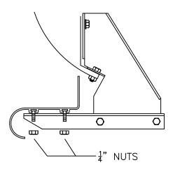
FOR PLASTIC BOARDS, APPLY FOAM TAPE AND STEP TREAD TO BOARD.
