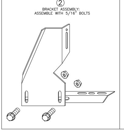
DEPENDING ON CAB STYLE, REMOVE RUBBER PLUGS AT MEASURED LOCATIONS AND INSTALL CLIP NUT AS SHOWN. OTHERS WIIL HAVE FACTORY MOUNTED NUTS AND WILL USE THE 8MM BOLT INCLUDED WITH THE BRACKETS.
