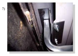
Attach the FL138 and CB41 assembly at the middle and rear bracket locations. Use one 5/16" bolt into the installed clip nut and 5/16" nuts on the installed bolts.
