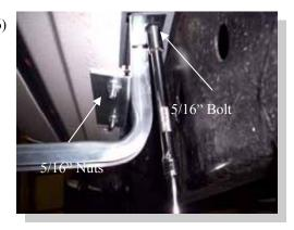
Attach the FL137 and CB40 assembly at the front bracket location. Use one 5/16" bolt into the installed clip nut and 5/16" nuts on the installed bolts.
