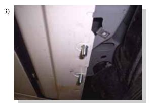
Insert one 5/16" flanged bolt through each factory hole along the pinch weld.
