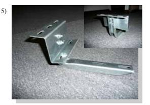
Assemble the FL138 and CB41 together using 5/16" nuts and bolts.
