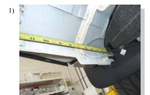
Measure from the front wheel well rearward. At locations 12", 34 1/2" and 63" is where the brackets will be attached. There are factory holes at these locations. Note: This photo is not of the Explorer.
