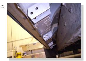
At the 12" location attach one FL113 using the removed factory bolts. Attach one FL114 at the other measured locations using factory bolts.
