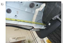
Measure from the front wheel well rearward. At locations 12", 34",56" and 73 1/2" is where the brackets will be attached. There are factory bolts at these locations, remove but do not discard.
