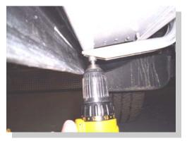
Place Driver side board on brackets so the board follows the contour of the body then level. Tighten all bolts in brackets and attach the board to the channels with 3/4" long self drilling screws.
