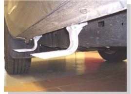
Attach channel brackets to mounting brackets with 5/16" bolts. Snug but do not tighten.
