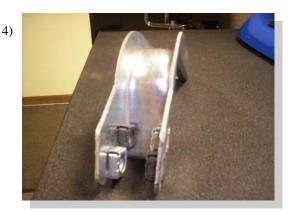
Insert Square clip nuts into channel brackets as shown.
