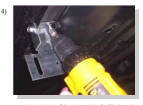
Attach FL136 at 8.5'' location with 5/16'' bolt and nut and 3/4'' long self drilling screw. At 27'', 40-1/2'' (21'', 37'' on driver side) and 60-1/2'' locations use FL135 bracket .
