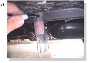
At measured locations hold the proper bracket in place and make a mark on the outside of the pinch weld and mark through the hole in the bracket.
