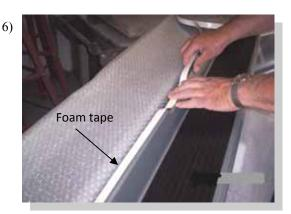
Apply foam tape to rear lip of board where it meets up with the vehicle. Apply step tread and logo now also. (Board in photo is not of the Highlander board)
