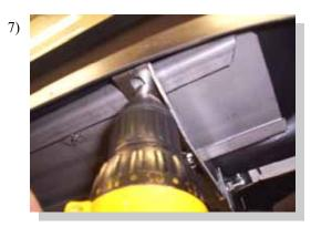
Place 67059P (Passenger) board on 3124F brackets, position board so it fits snug up against the vehicle and is level. Attach with 3/4" long self drilling screws through slots in the 3124F's into the steel plate under the board. Tighten bolts holding the 3124F 's to the flat brackets.
