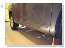
Attach one 3124F to each bracket using 5/16" bolts and nuts. Do not tighten. **ONLY THREE BRACKETS SHOWN IN PICTURE, YOU WILL HAVE FOUR BRACKETS PER SIDE.**
