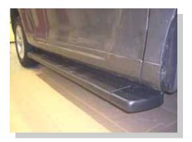
Repeat steps for driver side being sure to use the noted dimensions in step one for the driver side as they are different from the passenger side. Use 67059D board on drivers side.
