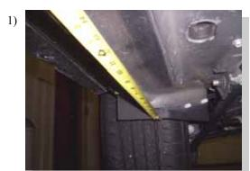
Measuring from the front of the REAR wheel well, measure towards the front of the vehicle. At locations 8.5", 27", 40-1/2" and 60-1/2" (8.5", 21", 37" and 60-1/2" Driver Side), make a mark on the pinch weld. You may have to move a bracket left or right
