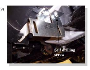
At 67 1/2" location drill a 23/64" hole through pinch weld. Attach FL131 using a 5/16" bolt and 3/4" long self drilling screw.
