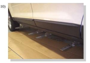
Attach a 3124F angle bracket to each flat bracket with 5/16" bolts and nuts. Do not tighten at this time.
