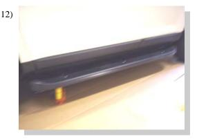
Position board on brackets keeping the rear edge of the board flush with the rear wheel opening to allow for optional front mud flaps. Have another person help hold the board or hold in place with small jacks.
