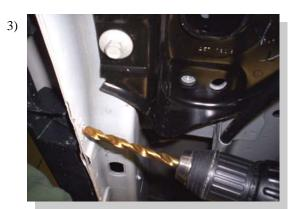
Drill a 23/64" hole through the pinch weld at the 9 1/2" location.
