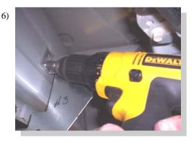
At 29" location drill a 23/64" hole in pinch weld and attach with 5/16' bolt and nut. Use a 3/8" nut driver and fasten BT41 bracket with 3/4" long self drilling screws. Tighten all bolts.
