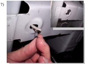
At 38 1/12" location dril 23/64" hole in pinch weld. Insert in-pull nut into factory slot in the underbody cross member. Fold metal tab flat to hold in place.
