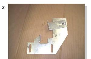
Assemble FL133 and BT41 with 5/16" bolt and nut. Leave BT41 loose until step #6.
