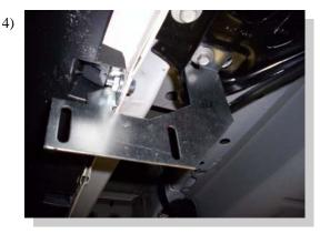
Attach FL134 bracket using the previously removed bolt and a supplied 5/16" bolt and nut.
