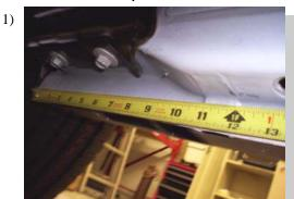
Measure from the front edge of the rear wheel well forward. At locations 9 1/2", 29",38 1/2" and 67 1/2" is where the brackets will be attached. There are notches in the factory trim at these locations.
