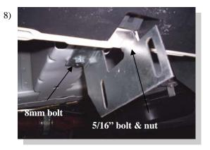
Attach FL132D (DRIVER) using a 5/16" bolt and nut to the pinch weld and supplied 8mm bolt into the in-pull nut.
