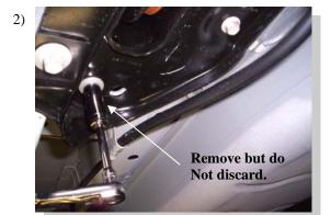
At the 9 1/2" location remove the factory bolt next to the slotted hole in the rear suspension bracket. *Do not discard bolt.*
