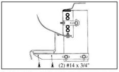
9. Use #14 x 3/4" self-drilling screws to fasten GlaStep to step supports, then tighten all bolts to 18 foot pounds
