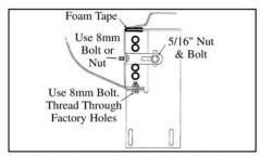
5. Place foam tape at top of FL130 flat plate. Bolt to AS02 then to pinch weld with 8mm bolts. Note: top of flat plate must hit rocker panel. Tighten to AS02 and 8mm bolt before tightening to pinch weld.
