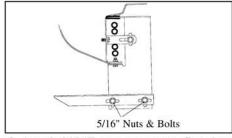
Attach 3124F step support to flat plate using two 5/16" nuts and bolts. Do not tighten at this time.
