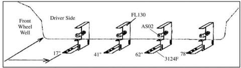
**3. Measure** from front wheel well, back 17", 41", 62", and 78". Mark these bracket locations. Note: Steel plates have been inserted under fiberglass to mount brackets securely using self-drilling screws. Note: Factory holes should be close to these measurements -- Use factory holes only.
