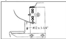
8. Position board on brackets adjusting bracket for a good fit. Use #12 x 1-1/4" self-drilling screws with rubber washers to attach lip of board to rocker panel.
