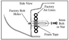
4. On passenger side with air and heat lines, wrap AS02 angled strap with foam tape so that lines are protected. Attach AS02 with 8mm bolts or nut to factory bolt holes on passenger and driver sides. Do not tighten at this time.
