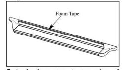
Apply foam tape to top edge of GlaStep. Remove protective strip from top edge of foam tape.
