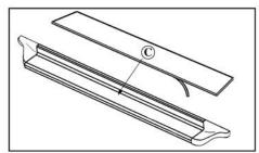
10. Tighten step support bolt and nut to 18 foot pounds. Place pad on step. Peel off tape backing to secure. Don't forget the Owens label!
