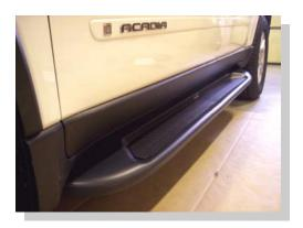
Repeat steps for passenger side. Use 67057P or 67061P board on passenger side.
