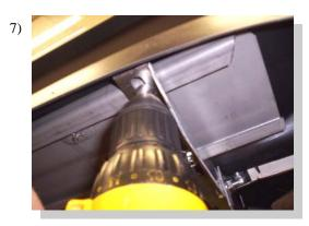
Place 67057D or 67061D (driver) board on 3124F brackets, position board so it fits snug up against the vehicle and is level. Attach with 3/4" long self drilling screws. Tighten bolts holding the 3124F 's to the flat brackets.
