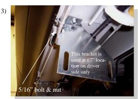
Attach FL128 bracket at 67" location on driver side only with 5/16" bolt and nut and one 3/4" long self drilling screw. Pre drill hole for self taping screw with 1/8" drill bit.
