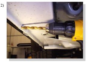
At each mark drill a 23/64" hole through the pinch weld.
