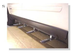
Attach one 3124F to each bracket using 5/16" bolts and nuts. Do not tighten.
