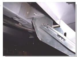
Attach one channel bracket with 5/16 bolts and nuts on each flat bracket. Snug but do not tighten.
