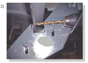
Attach an FL125 with supplied 5/16 bolt and nut through hole where cable bracket was removed. Drill a 5/16" hole from the back side of the pinch weld to line up with the hole in the bracket and attach with 5/16" bolt and nut.
