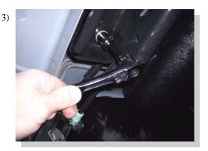
Remove the two forward bolts of the rear leaf spring holder. Do not discard, these will be used to attach rear bracket.
