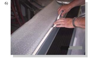
Attach foam tape to the top lip of the board where it meets up with the body. Attach step tread and logo also.
