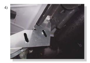
Attach FL127D using bolts removed in step3. From back side of pinch weld drill 5/16" hole through pinch weld to line up with the hole in the bracket . Insert a 5/16" bolt and fasten with nut . Tighten all bolts.
