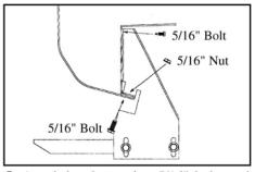
**5.** Attach brackets using 5/16" bolts and nuts through pinch weld holes. Use 5/16" bolts for installed clip nuts.
