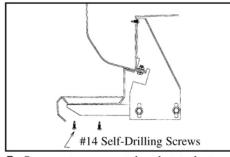
7. Secure step support bracket to bottom of board using two #14 x 3/4" self-drilling screws per bracket. **Tighten all bolts to 18 foot pounds.**
