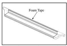
**6.** Apply foam tape strips to top edge of running board.
