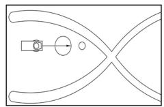
**3.** Remove plastic plug from underbody at measured locations and install clip nut as shown.
