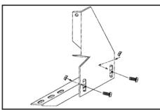
**4.** Assemble FL119 to 3124F using two 5/16" nuts and bolts. **Do not tighten at this time.**
