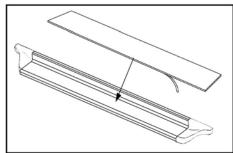
8. Place step pad on step area. Peel off tape backing to secure. Don't forget the Owens logo!
