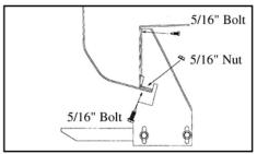
**5.** Attach brackets using 5/16" bolts and nuts through pinch weld holes, and 5/16" bolt into installed clip nut.
