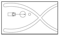
Remove plastic plug from underbody at measured locations and install clip nut as shown.
