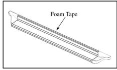
**6.** Apply foam tape strips to top edge of running board.
