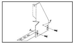
**4.** Assemble FL119 to 3124F using two 5/16" nuts and bolts. **Do not tighten at this time.**
