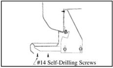
7. Secure step support bracket to bottom of board using #14 x 3/4" self-drilling screws. Tighten all bolts to 18 foot pounds.
