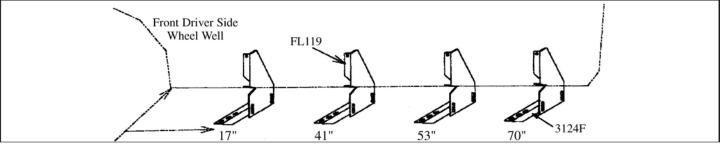
2. Measure from front wheel well, back 17", 41", 53" and 70". Mark these bracket location centers. Note: Steel plates have been installed under stepping area to mount brackets securely using self-drilling screws.
