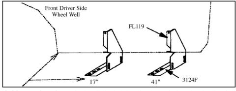
**3. Measure** from front wheel well, back 17" and 41". Mark these bracket location centers. Note: Steel plates have been inserted under fiberglass to mount brackets securely using self-drilling screws.
