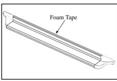
**7.** Apply foam tape strips to GlaStep edge.
