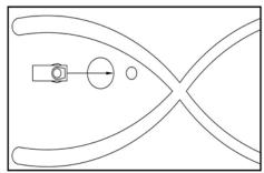
Remove plastic plug from underbody at all measured locations and install clip nut as shown.
