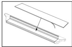
9. Place step pad on GlaStep. Peel off tape backing to secure. Don't forget the Owens logo!
