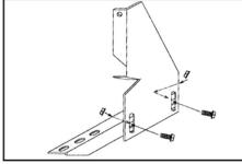
5. Assemble FL119 to 3124F using two 5/16" nuts and bolts. **Do not tighten at this time.**
