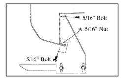
**6.** Attach brackets using 5/16" bolts and nuts through pinch weld holes, and 5/16" bolts into clip nuts.
