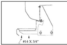
8. Secure step support bracket to bottom of GlaStep using two #14 x 3/4" self-drilling screws per bracket. Tighten all bolts to 18 foot pounds.
