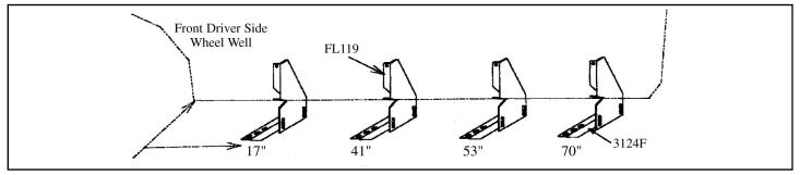
**3. Measure** from front wheel well, back 17", 41", 53" and 70". Mark these bracket location centers. Note: Steel plates have been inserted under fiberglass to mount brackets securely using self-drilling screws.
