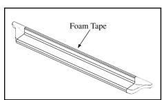
**7.** Apply foam tape strips to GlaStep edge.
