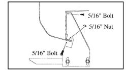
**6.** Attach brackets using 5/16" bolts and nuts through pinch weld holes, and 5/16" bolts into clip nuts.
