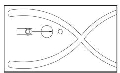
**4.** Remove plastic plug from underbody at all measured locations and install clip nut as shown.
