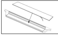
9. Place step pad on GlaStep. Peel off tape backing to secure. *Don't forget the Owens label!*
