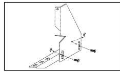
**5.** Assemble FL119 to 3124F using two 5/16" nuts and bolts. **Do not tighten at this time.**
