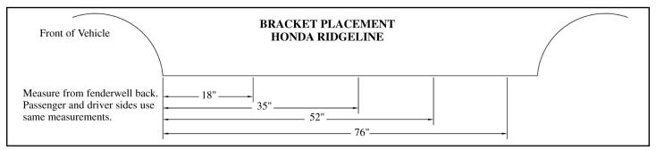
3. At measured bracket locations, remove plastic plugs from factory holes in frame and underbody. This is where brackets will be bolted.
