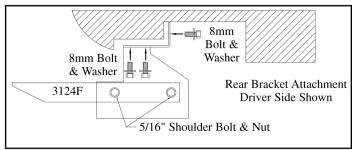
**5.** Attach FL118D to driver side rear bracket location and tighten. Attach 3124F angle to FL118D, but do not tighten at this time.
