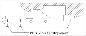
**6.** Position board on brackets and attach with self-drilling screws. **Tighten all bolts** not previously tightened.
