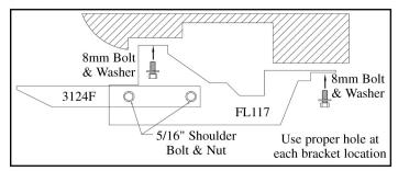
**4.** Bolt FL117 bracket to the three forward bracket locations and tighten. Attach 3124F angle to FL117 but do not tighten at this time.
