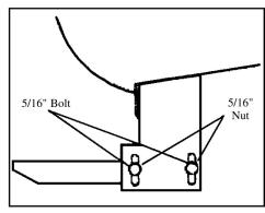
5. Use two 5/16" nuts & bolts to secure 3124F step support to FL50. Snug, but do not tighten at this time.
