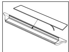
Tighten step support bolt and nut to 18 foot pounds. Place pad on step. Peel off tape backing to secure. Don't forget the Owens label!
