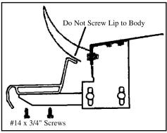
7. Center board between wheel wells on brackets attached to vehicle. Screw step to support bracket with two #14 x 3/4" self-drilling screws per bracket. Do not fasten lip of board to vehicle body.
