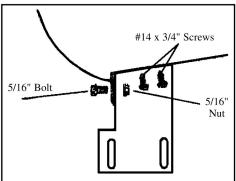
3. Measure from front wheel well, back 4. Place flat bracket FL103 against the pinch weld at the locations show above. Drill a 5/16" hole through the pinch weld if factory hole is not there. Mount the flat bracket to the pinch weld with 5/16" nut and bolt. Finish by putting two #14 x 3/4" screws through flat bracket into rocker panel.
