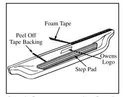
6. Apply foam tape to top edge of running board. Remove protective strip from top edge of foam tape.
