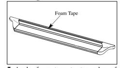
**7.** Apply foam tape to top edge of GlaStep. Remove protective strip from top edge of foam tape.
