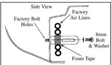
**4.** On passenger side with air and heat lines, wrap AS02 angled strap with foam tape so that lines are protected. Attach AS02 with 8mm bolts and lock washers to factory bolt holes on passenger and driver sides. **Do not tighten at this time.**
