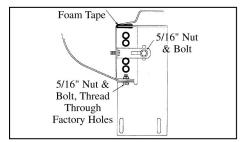
5. Place foam tape at top of FL29 flat plate. Bolt to AS02 then to pinch weld with 5/16" nuts and bolts. Note: top of flat plate must hit rocker panel. Tighten FL29 to AS02 and 8mm bolt before tightening to pinch weld.
