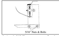
**6.** Attach 3124F step support to flat plate using two 5/16" nuts and bolts. **Do not tighten at this time.**
