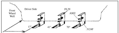
**3. Measure** from front wheel well, back 17", 41", and 70". Mark these bracket locations. Note: Steel plates have been inserted under fiberglass to mount brackets securely using self-drilling screws. Note: Factory holes should be close to these measurements -- Use factory holes only.
