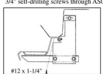
7. Secure GlaStep to body with #12 x 1-1/4" self-drilling screws with rubber washers.
