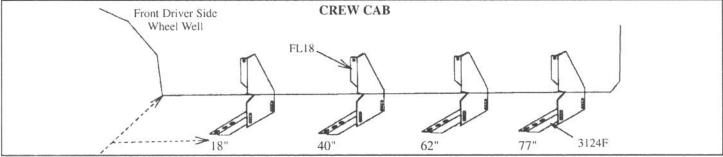
3. Measure from front wheel well, back to dimensions shown above. Mark these bracket location centers.
