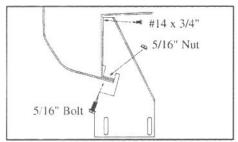
4. Drill 5/16"" diameter hole through pinch weld at marks. Bolt FL18 flat bracket to pinch weld with 5/16" x 3/4" bolt and nut, then use #14 x 3/4" self-drilling screw in top hole into rocker panel.
