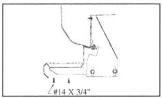
8. Secure step support bracket to bottom of board using two #14 x 3/4" self-drilling screws per bracket. Tighten all bolts to 18 foot pounds.
