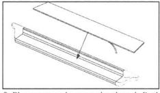
9. Place step pad on running board. Peel off tape backing to secure. Don't forget the Owens label!
