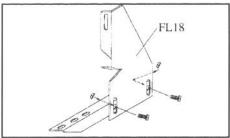
Attach 3124F to FL18 using two 5/16" washer head bolts with nuts. Snug, but do not tighten at this time.
