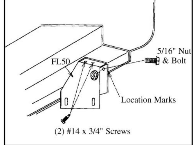
marks. Attach FL50 bracket with 5/16" nut & bolt, then use two #14 x 3/4" selfdrilling screws to secure top of FL50.
