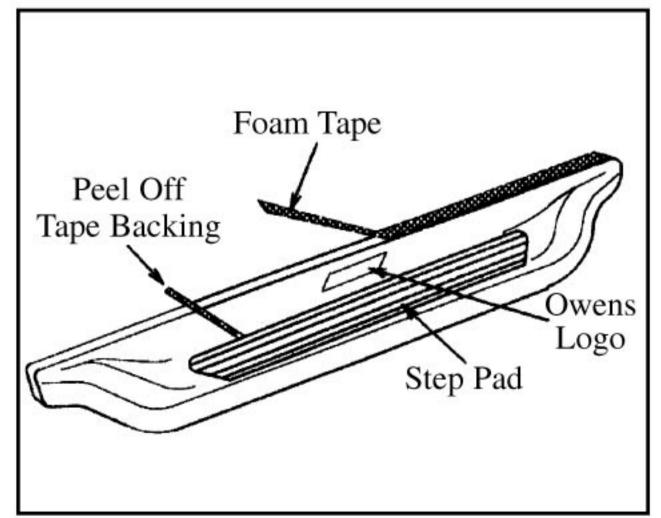
8. Apply foam tape to top edge of running boad. Remove protective strip from top edge of foam tape.
