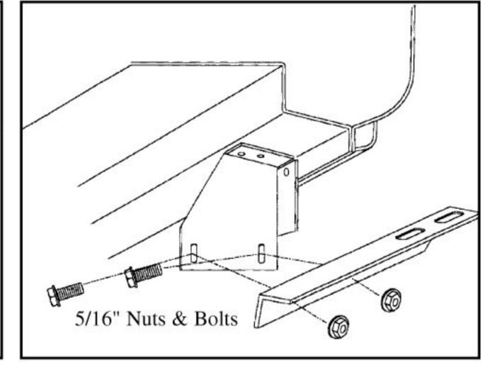
5. Use two 5/16" nuts & bolts to secure 3124F step support to FL50. Snug, but do not tighten at this time.
