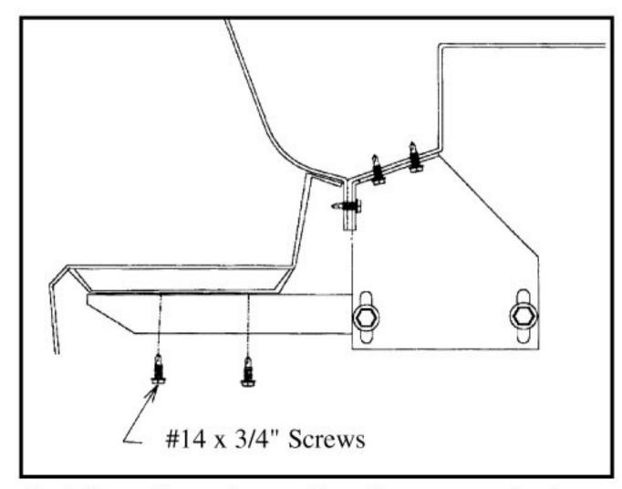
9. Align board on brackets attached to vehicle. Screw step to support bracket with two #14 x 3/4" self-drilling screws per bracket. Do not fasten lip of board to vehicle body.
