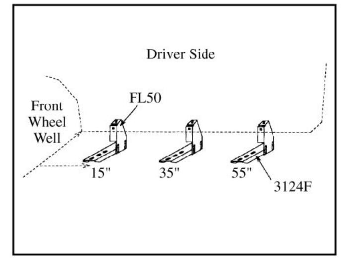
3. Measure from front wheel well, back 15", 4. Drill 5/16" diameter hole in pinch weld at 35" and 55". Mark these bracket locations.
