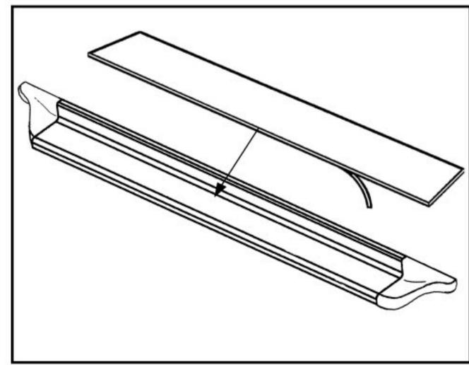
10. Tighten step support bolt and nut to 18 foot pounds. Place pad on step. Peel off tape backing to secure. Don't forget the Owens label!
