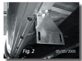
2. Attach brackets to rear side of pinch weld with 5/16" bolt & nut. On bracket being placed at factory holes, slightly bend tab on bracket forward and place tab on front side of pinch weld. (see Fig. 2)
