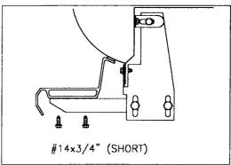
6. Position step on brackets and tight to truck body Secure step support bracket to bottom of Glastep using two #14 x 3/4" self-drilling screws (SHORT) per bracket. Repeat for all brackets. DO NOT USE LONG SELF TAPPERS UNDER THE BOARD!
