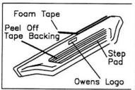
Clean surface prior to attaching tape and step pads with denatured alcohol. Apply foam tape to top lip of board. Position step pad on stepping surface. Peel off tape backing starting with the rear strip. Keep pad in position, peel off backing then apply pressure to top of pad to to stick tape to board. Continue above steps for all tape strips.
