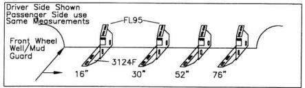
Measure from the wheel well, back to the dimensions shown above. Mark these bracket location centers. The 1st bracket uses self drilling screws, the others locations use factory mounting screws. Note: Steel plates have been inserted under fiberglass to mount brackets.
