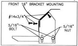
4. Use 2 self drilling screws to mount FL95 to the pinch weld. Use 1 self drilling screw to attach into the rocker panel. Attach support 3214F to FL95 using 2 5/16" bolts and nuts.
