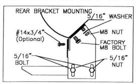
5. Remove the factory M8 bolt, reinstall mounting the FL95 bracket. Use a 5/16" washer and M8 Nut on the exposed stud. Attach support 3214F to FL95 using 2 5/16" bolts and nuts.
