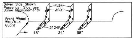
3. Measure from the wheel well, back to the dimensions shown above. Mark these bracket location centers. Note: Steel plates have been inserted under fiberglass to mount brackets. Double check your marks to be sure they line up with the steel plates before drilling. Also there are many holes, USE THE RIGHT ONES!
