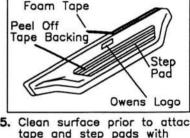
5. Clean surface prior to attaching tape and step pads with denatured alcohol. Apply foam tape to top lip of board. Position step pad on stepping surface. Peel off tape backing starting with the rear strip. Keep pad in position, peel off backing then apply pressure to top of pad to stick tape to board. Continue above steps for all tape strips.
