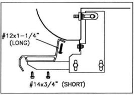
6. Position step on brackets and tight to truck body. Screw step to truck with #12 x 1-1/4" self-drilling screws with rubber washers (LONG), three per side. Secure step support bracket to bottom of GlaStep) using two #14 x 3/4" self-drilling screws (SHORT) per bracket. Repeat for all Brackets. DO NOT USE LONG SELF TAPPERS UNDER THE BOARD!
