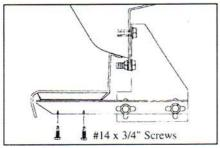
8. Secure bracket to step with two #14 x 3/4" self-drilling screws per bracket. Tighten all bolts to 18 foot pounds.
