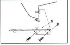
5. Attach 3124F step supports to FL11 6. Apply foam tape strips to top step edge. using 5/16" washer head bolts and nuts.
