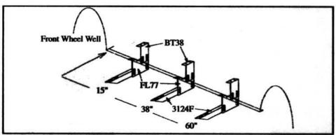
Measure from front wheel well, back to dimensions shown above. Mark these bracket location centers.
