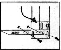
5. Assemble FL77 to 3124F using two 5/16" nuts and bolts. Do not tighten at this time.
