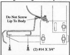
Secure step support bracket to bottom
