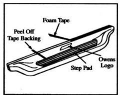
6. Clean surface prior to attaching tape and step pads with denatured alcohol. Apply foam tape to top lip of board. Position step pad on stepping surface. Peel off tape backing starting with rear strip. Keep pad in position, peel off backing then apply pressure to top of pad to stick tape to board. Continue above steps for
