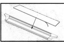
9. Place step pad on board. Peel off tape backing to secure. Don't forget the Owens label!
