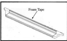
Apply foam tape strips to running board edge.
