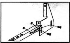
4. Assemble FL39 to 3124F using two 5/16" nuts and bolts. Do not tighten at this time.
