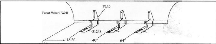
3. Measure from front wheel well, back 181/2", 40" and 64". Mark these bracket location centers.
