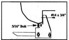
5. Drill 5/16"" diameter hole through pinch weld at marks. Bolt FL39 flat bracket to pinch weld with 5/16" x 3/4" bolt and nut, then use #14 x 3/4" self-drilling screw in top hole into rocker panel.
