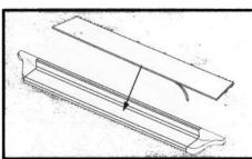
8. Place step pad on running board. Peel off tape backing to secure. Don't forget the Owens label!
