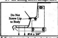
Position running board on brackets and tight to truck body. Screw board to bracket using two #14 x 3/4" selfdrilling screws per bracket. Tighten all
