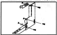
Assemble bracket components with 5/16" nuts & bolts as shown. Do not tighten at this time.
