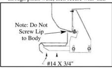
8. Position running board on bracket and tight to truck body. Do not fasten lip to body. Screw board to bracket using two #14 x 3/4" self-drilling screws per bracket. Tighten all bolts to 18 foot pounds.
