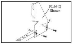
Attach 3124F to FL46 using two 5/16" washer head bolts with nuts. Snug, but do not tighten at this time.
