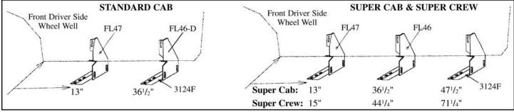
3. Measure from front wheel well, back to dimensions shown above. Mark these bracket location centers.
