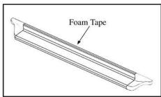
Apply foam tape to top edge of running board. Remove protective strip from top edge of foam tape.
