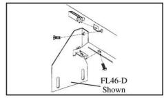
6. Find 5/16" diameter holes in pinch weld at rear mark, then attach bent tab using 5/16" washer head bolts with nuts. Secure top of bent tab to rocker panel using 5/16" clip nut in factory locations.
