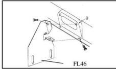
5. At first mark, find factory bolt hole in pinch weld. Remove rubber cover from access hole. Place 5/16" clip nut in line with top bolt hole, insert 5/16" bolt through bracket and factory hole, then into nut. Finish with bolt up through pinch weld, then secure with nut.
