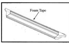
Apply foam tape strips to running board edge.
