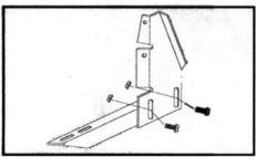
4. Assemble FL15 to 3124F using two 5/16" nuts and bolts. Do not tighten at this time.
