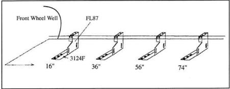
Measure from front wheel well, back to dimensions shown above. Mark these bracket location centers.
