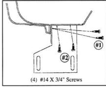
4. Use four #14 x 3/4" screws to attach FL87. Use Caution: Sheet metal is thin. Do not over tighten.
