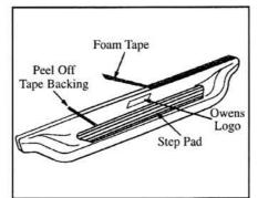
6. Clean surface prior to attaching tape and step pads with denatured alcohol. Apply foam tape to top lip of board. Position step pad on stepping surface. Peel off tape backing starting with rear strip. Keep pad in position, peel off backing then apply pressure to top of pad to stick tape to board. Continue above steps for all tape strips.
