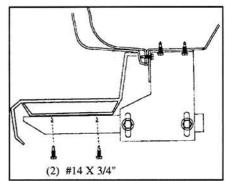
Secure step support bracket to bottom of GlaStep using two #14 x 3/4" selfdrilling screws per bracket. Tighten all bolts to 18 foot pounds.
