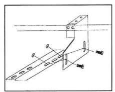
Assemble bracket components with 5/16" nuts and bolts as shown. Do not tighten at this time.
