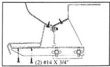
Secure step support bracket to bottom of GlaStep using two #14 x 3/4" selfdrilling screws per bracket. Tighten all bolts to 18 foot pounds.
