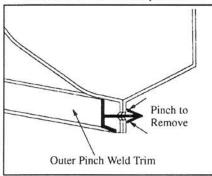
Remove the factory pinch weld trim. Pinch the plastic clips to remove.
