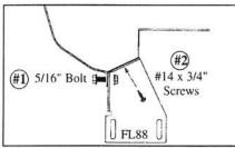
At marked factory holes, bolt FL88 to pinch weld using 5/16" nuts and bolts, then use #14 x 3/4" self-drilling screws to secure top of FL88 to inner panel.
