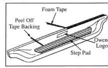
7. Clean surface prior to attaching tape and step pads with denatured alcohol. Apply foam tape to top lip of board. Position step pad on stepping surface. Peel off tape backing starting with rear strip. Keep pad in position, peel off backing then apply pressure to top of pad to stick tape to board. Continue above steps for all tape strips.
