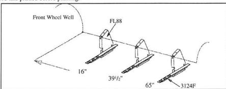
4. Measure from front wheel well, back 16", 39<sup>1</sup>/<sub>2</sub>"" and 65". Mark these bracket location centers. Note: Steel plates have been inserted under fiberglass to mount brackets securely using self-drilling screws.
