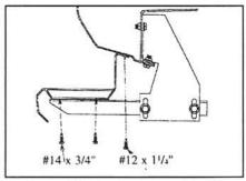
Secure GlaStep to body with #12 x 1<sup>1</sup>/<sub>4</sub>" self-drilling screws with rubber washers. Secure step support bracket to bottom of GlaStep using two #14 x 3/4" self-drilling screws per bracket. Tighten all bolts to 18 foot pounds.
