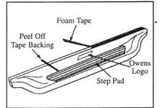
6. Clean surface prior to attaching tape and step pads with denatured alcohol. Apply foam tape to top lip of board. Position step pad on stepping surface. Peel off tape backing starting with rear strip. Keep pad in position, peel off backing then apply pressure to top of pad to stick tape to board. Continue above steps for all tape strips.
