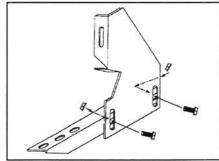
Assemble FL83 to 3124F using two 5/16" nuts and bolts. Do not tighten at this time.
