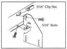
Find 5/16" holes in pinch weld at 33<sup>1</sup>/<sub>2</sub>" and 64" marks. Secure top of FL83 to rocker panel using 5/16" clip nut in factory locations.
