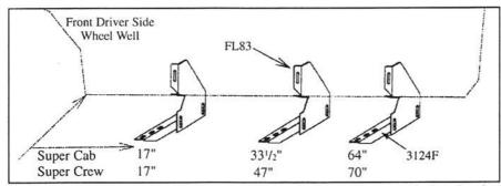
Measure from front wheel well, back to locations shown above. Mark these bracket location centers. Note: Steel plates have been inserted under fiberglass to mount brackets securely using self-drilling screws.
