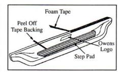
6. Clean surface prior to attaching tape and step pads with denatured alcohol. Apply foam tape to top lip of board. Position step pad on stepping surface. Peel off tape backing starting with rear strip. Keep pad in position, peel off backing then apply pressure to top of pad to stick tape to board. Continue above steps for all tape strips.
