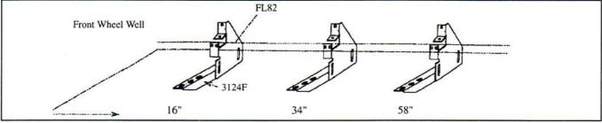
3. Measure from front wheel well, back to dimensions shown above. Mark these bracket location centers.
