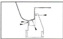
4. Use four #14 x 3/4" screws to attach FL82. Use Caution: Sheet metal is thin. Do not over tighten.
