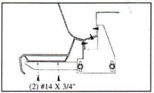
8. Secure step support bracket to bottom of GlaStep using two #14 x 3/4" selfdrilling screws per bracket. Tighten all bolts to 18 foot pounds.
