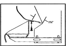
8. Position step on bracket aligning step with cab step. Attach to box using 3 front, rear and center #12 x 1-1/4" self-drilling screws with rubber washers.
