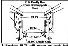
4. Attach flat plates #FL73 to box supports. Align front of plate with box support. Use one #14 x 3/4" self-drilling screw to attach rear of FL73, drill 5/16" hole through front hole of FL73 in box support. Insert clip nut and secure with 5/16" bolt.
