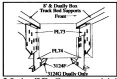
3. Brackets FL73 will mount on truck bed supports as shown.
