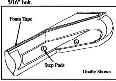
7. Clean surface prior to attaching tape and step pads with denatured alcohol. Apply foam tape to back of step where it mates with body. Place step pad on GlaStep. Peel off tape
