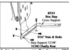
6. Attach step support to flat plate using 5/16" nuts and bolts. Do not tighten at this time. Attach cross support BT43 as shown. Use 3124G for dually rear only.
