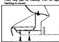
9. Attach GlaStep to bracket using two #14 x 3/4" self-drilling screws per support. Adjust height of step, then tighten all bolts.
