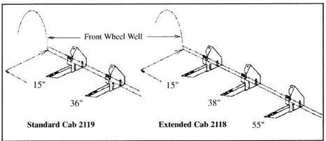
3. Measure from front wheel well. Note: Steel plates have been inserted under fiberglass to mount brackets securely using self-drilling screws.
