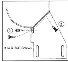
4. Use #14 x 3/4" screws to secure FL81flat bracket at marks on pinch weld.
