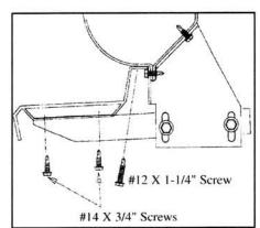
7. Secure GlaStep to body with #12 x 1-1/4" self-drilling screws with rubber washers. Secure step support bracket to bottom of GlaStep using two #14 x 3/4" self-drilling screws per bracket. Tighten all bolts to 18 foot pounds.
