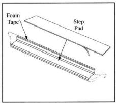
6. Apply foam tape strips to GlaStep edge. Place step pad on GlaStep. Peel off tape backing to secure. Don't forget the Owens label!
