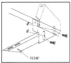
5. Assemble FL81 to 3124F using two 5/16" nuts and bolts. **Do not tighten at this time.**
