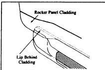
8A. Place GlaStep on bracket, Note that riser lips on end of board are to be flush behind rocker cladding on 2131.
