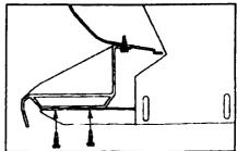
9. Attach GlaStep to bracket using two #14 x 3/4" self-drilling screws per support. Adjust height of step, then tighten IN178B 12/13/04
