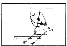
Attach 3124F step supports to FL78 (or FL79) flat brackets using 5/16" bolts and nuts. Do not tighten at this time.
