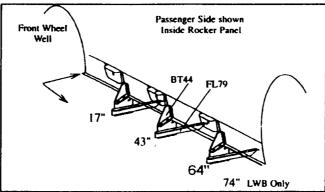
Measure from front wheel well to factory bracket hole locations shown above. Find these factory bracket locations.
