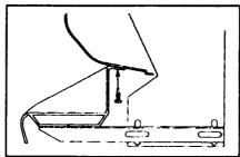
8B, Position step on bracket aligning step with cab step. Attach to box using 3 front, rear and center #12 x 1-1/4" self-drilling screws with rubber washers.
