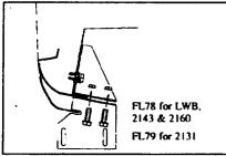
Bolt FL78 (or FL79) to BT44 using two 5/16\* nuts & bolts. Then tighten all three bolts to 18 foot pounds.
