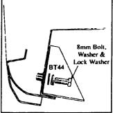
J. Mount BT44 flat bracket to body using 8mm bolts in factory holes at noted locations. Do not tighten at this time.
