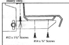
11. Position step on bracket. Secure with #12 x 1-1/4" self-drilling screws. Tighten all bolts to 18 foot pounds.
