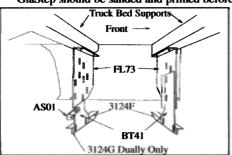
3. Brackets FL73-D&P will mount on truck bed supports as shown at right.
