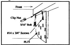
4. Attach flat plates #FL73 to box supports. Align front of plate with box support. Use one #14 x 3/4" self-drilling screw to attach rear of FL73, drill 5/16" hole through front hole of FL73 in box support. Insert clip nut and secure with 5/16" bolt.
