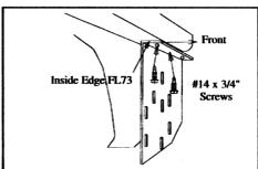
5. Attach FL73 to rear bed support using two #14 x 3/4" screws. Align inside edge of FL73 with inside of front FL73.
