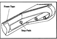
7. Clean surface prior to attaching tape and step pads with denatured alcohol. Apply foam tape to top lip of board. Position step pad on stepping surface. Peel off tape backing starting with rear strip. Keep pad in position, peel off backing then apply pressure to top of pad to stick tape to board. Continue above steps for all tape strips.
