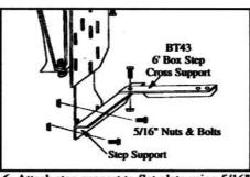
6. Attach step support to flat plate using 5/16" nuts and bolts. Do not tighten at this time. For 6' Box Only: Attach cross support BT43 as shown.
