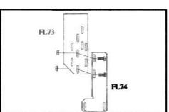
5. Bolt FL74 to FL73 using two 5/16" nuts and bolts in slots shown.
