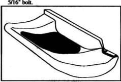
7. Clean surface prior to attaching tape and step pads with denatured alcohol. Apply foam tape to back of step where it mates with body. Place step pad on GlaStep. Peel off tape
