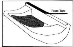
7. Clean surface prior to attaching tape and step pads with denatured alcohol. Apply foam tape to back of step where it mates with body. Place step pad on GlaStep. Peel off tape backing to secure.
