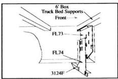
Brackets FL73 will mount on truck bed supports as shown.
