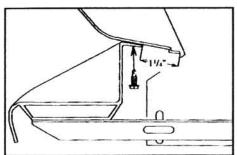
8. Position step on bracket aligning step with cab step (keep back lip of box step approximately 1-1/4" from box lip). Attach to box using 3 front, rear and center #12 x 1-1/4" self-drilling screws with rubber washers.
