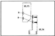
Bolt FL74 to FL73 using two 5/16" nuts and bolts in slots shown.
