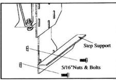
Attach step support to flat plate using 5/16" nuts and bolts. Do not tighten at this time.
