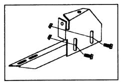
4. Assemble FL67 to 3124F using two 5/16" nuts and bolts. Do not tighten at this time.
