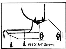
8. Secure step support bracket to bottom of GlaStep using two #14 x 3/4" self-drilling screws per bracket. Tighten all bolts to 18 foot pounds.
