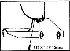
Secure GlaStep to body with #12 x 1-1/4" self-drilling screws with rubber washers.
