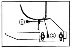
5. Use #14 x 3/4" screws to secure FL67 flat bracket at marks on pinch weld.
