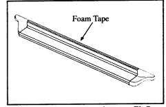
**6.** Apply foam tape strips to GlaStep edge.
