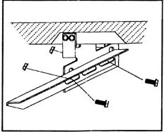
5. Assemble FL68 to 3124F using two 5/16" nuts and bolts. Do not tighten at this time.
