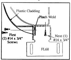
4. Position FL68 flat bracket at marks on pinch weld. From front, use two #14 x 3/4" self-drilling screws to fasten to pinch weld. Next, use one #14 x 3/4" to fasten FL68 to bottom of rocker panel.
