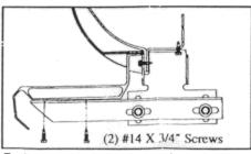
7. Secure step support bracket to bottom of GlaStep using two #14 x 3/4" self-drilling screws per bracket. Tighten all bolts to 18 foot pounds.
