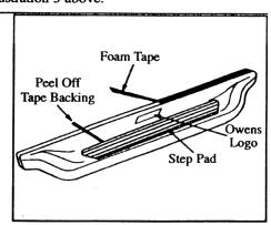
6. Clean surface prior to attaching tape and step pads with denatured alcohol. Apply foam tape to top lip of board. Position step pad on stepping surface. Peel off tape backing starting with rear strip. Keep pad in position, peel off backing then apply pressure to top of pad to stick tape to board. Continue above steps for all tape strips.
