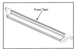
**6.** Apply foam tape strips to top GlaStep edge.
