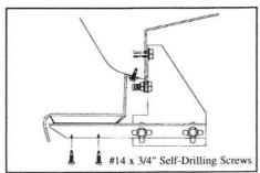
8. Secure bracket to GlaStep with two #14 x 3/4" self-drilling screws per bracket. Tighten all bolts to 18 foot pounds.
