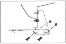
5. Attach 3124F step supports to FL11 using 5/16" washer head bolts and nuts.
