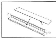
Place step pad on GlaStep. Peel off tape backing to secure. Don't forget the Owens label! IN-121 7/1/02
