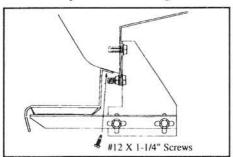
7. Position GlaStep to body and secure with three #12 x 1-1/4" screws with rubber washers per side.
