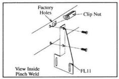
4. Mount brackets to body with 5/16" bolt and nuts, through existing holes in vehicle at marked locations. Use clip nuts in top holes. Do not tighten nuts.
