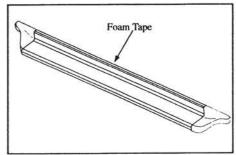
Apply foam tape strips to top GlaStep edge.
