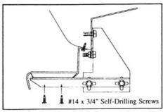
Secure bracket to GlaStep with two #14
