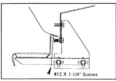
7. Position GlaStep to body and secure with three #12 x 1-1/4" screws with rubber washers per side.
