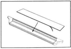
Place step pad on GlaStep. Peel off tape backing to secure. Don't forget the Owens label! IN\_110 7/1/02
