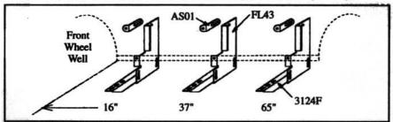
3. Measure from front wheel well, back 16", 37" and 65". Mark these bracket locations. Note: Steel plates have been inserted under fiberglass to mount brackets securely using self-drilling screws. Double check your marks to be sure they line up with
