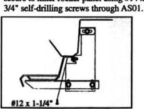
Secure GlaStep to body with #12 x 1-1/4" self-drilling screws with rubber washers.
