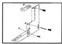
4. Assemble bracket components with 5/16" nuts & bolts as shown. Do not tighten at this time.
