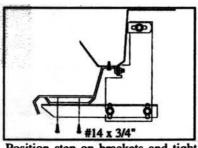
8. Position step on brackets and tight to truck body. Screw step to bracket using two #14 x 3/4" self-drilling screws per bracket and adjust GlaStep to body. Tighten all bolts to 18 foot pounds.
