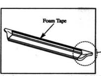
6. Apply 10am tape to top edge of GlaStep. Remove protective strip from top edge of foam tape.
