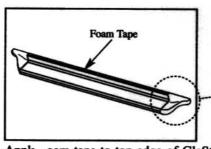
6. Apply 10am tape to top edge of GlaStep. Remove protective strip from top edge of foam tape.
