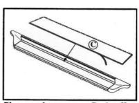
9. Place pad on step. Peel off tape backing to secure. Don't forget the Owens label!
