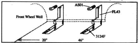
3. Measure from front wheel well, back 20" and 46". Mark these bracket locations. Note: Steel plates have been inserted under fiberglass to mount brackets securely using self-drilling screws. Double check your marks to be sure they line up with the steel plates before drilling.
