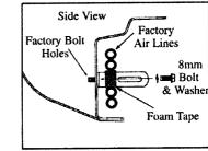
4. On passenger side with air and heat lines, wrap AS02 angled strap with foam tape so that lines are protected. Attach AS02 with 8mm bolts and lock washers to factory bolt holes on passenger and driver sides. **Do not tighten at this time.**
