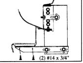
9. Use #14 x 3/4" self-drilling screws to fasten GlaStep to step supports, then tighten all bolts to 18 foot pounds
