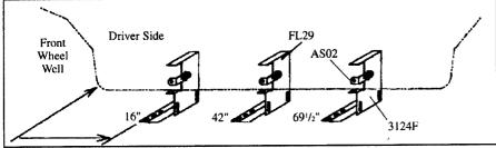
**3. Measure** from front wheel well, back 16", 42", and 69-1/2". Mark these bracket locations. Note: Steel plates have been inserted under fiberglass to mount brackets securely using self-drilling screws. Note: Factory holes should be close to these measurements -- Use factory holes only.
