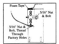
5. Place foam tape at top of FL29 flat plate. Bolt to AS02 then to pinch weld with 5/16" nuts and bolts. Note: top of flat plate must hit rocker panel. Tighten FL29 to AS02 and 8mm bolt before tightening to pinch weld. Note: On 2005 models, front and rear brackets attach using the factory stud and nut supplied in bolt kit.
