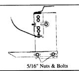
6. Attach 3124F step support to flat plate using two 5/16" nuts and bolts. Do not tighten at this time.
