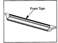
7. Apply foam tape to top edge of GlaStep. Remove protective strip from top edge of foam tape.
