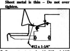
Screw step to truck with #12 x 1-1/4" self-drilling screws with rubber washers (K), three per side.
