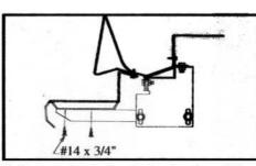
9. Screw step to bracket using two #14 x 3/4" self-drilling screws per bracket. Tighten all bolts to 18 foot pounds.
