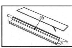
10. Place pad on step. Peel off tape backing to secure. Don't forget the Owens label!
