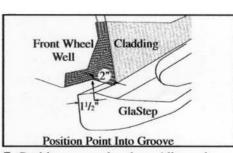
7. Position step on brackets. Align point on GlaStep into groove of cladding.
