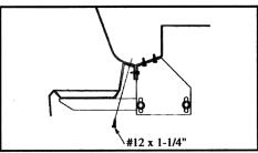
8. Position GlaStep on brackets, then using three #12 x 1-1/4" screws with rubber washers, attach step to rocker panel at fender flare intersection front and back,
