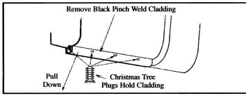
3. Remove the plastic pinch weld cover cladding from bottom of rocker panel.
