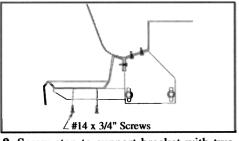
9. Screw step to support bracket with two #14 x 3/4" self-drilling screws per bracket.
