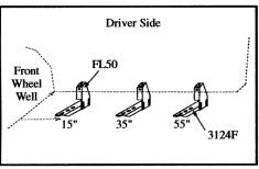
5. Measure from front wheel well, back 15", 6. Drill 5/16" diameter hole in pinch weld at 35" and 55". Mark these bracket locations.
