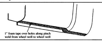
4. Adhere black foam tape onto vehicle to cover the "Christmas Tree" holes. Start at front wheel well over fender flares, along pinch weld, then over rear fender flare.
