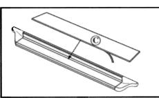
10. Tighten step support bolt and nut to 18 foot pounds. Place pad on step. Peel off tape backing to secure. Don't forget the Owens label!
