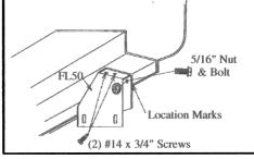
marks. Attach FL50 bracket with 5/16" nut & bolt, then use two #14 x 3/4" selfdrilling screws to secure top of FL50.
