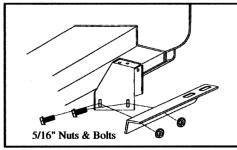
7. Use two 5/16" nuts & bolts to secure 3124F step support to FL50. Snug, but do not tighten at this time.
