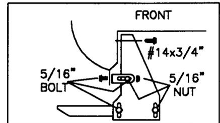
3. Measure from the wheel well, back to the dimensions shown above. Mark these bracket location centers. Note: Steel plates have been inserted under fiberglass to mount brackets securely using self drilling screws. Double check your marks to be sure they line up with the steel plates before drilling.
