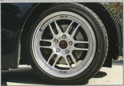
We conclude this upgrade update with a review of the new shoes and soles on our AP2, starting first with coveted 17x7.5 Enkei RPF1 rims tucked in each wheelwell. The RPF1's weigh a remarkable 15.2 pounds each, primarily because of Enkel's MAT process, a method for producing light, strong cast wheels by spinning the castings during manufacture to compress the metal.
