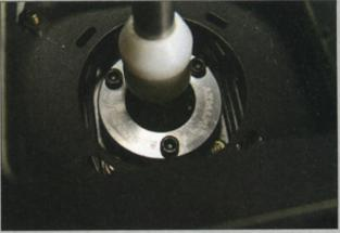
There's a marked knob height difference with the new shaft, but the shifting has also become far more precise with the Axialflow. It definitely puts the driver in much more intimate contact with the gearbox. The only issue we have happens at high revs, when a crazy amount of vibration comes up through the shaft. Paul has a fix for this though, essentially a rubber boot included with his latest versions of the kit.
